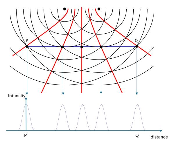
The maxima are not uniformly separated. This is because we are too close to the sources. We drew all maxima to have the same intensity. In reality this cannot be the case since the distances from the sources are different so the intensity must be dropping as we move away from the central maximum in either direction.
