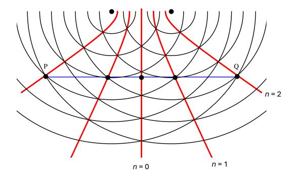
The hyperbolas intersect the blue line joining P and Q at the points shown by dots. These are points of maximum intensity.
